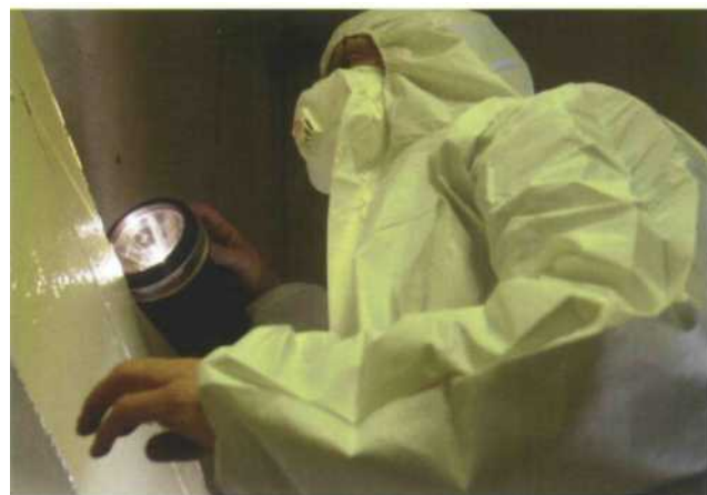
Figure 7.24 A torch being used to illuminate fine settled dust
