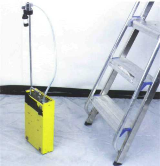
Figure 7.27 Air sampling during clearance
