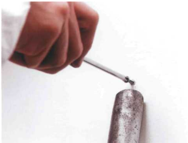
Figure 7.6 Drilling using a low-speed drill with cowl and fitted with LEV
