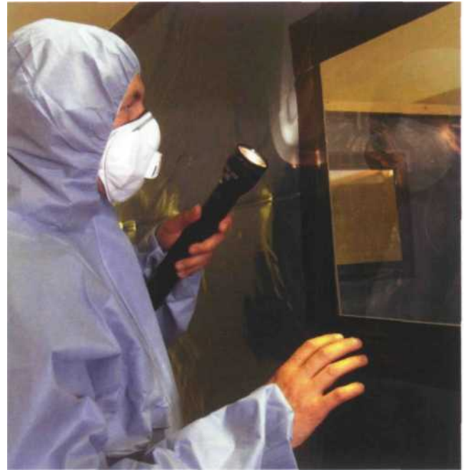
Figure 6.18 A torch being used to find smoke leaks
